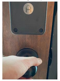
5. With the lock in the locked position, the <u>egress button</u> (green unlocking only button) can be tested by pressing the green button to see if the lock actuates to an unlocked position.
